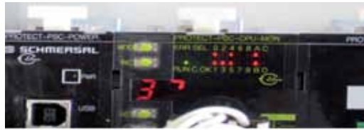
Fig. 9: Clear display on the CPU module of which input and output signals connected
